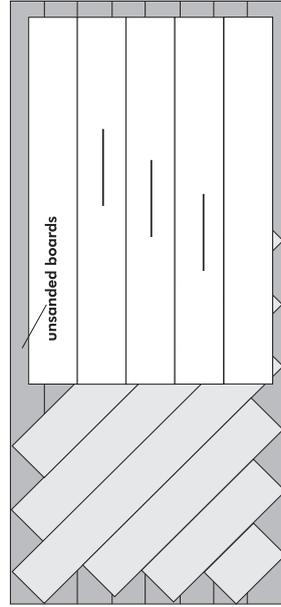
**Plank and Strip Floors** - sand in the direction the boards are laid, with the wood grain.
